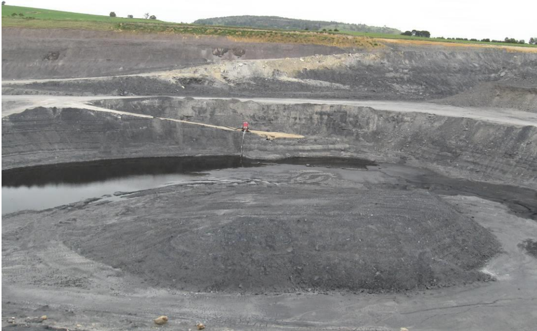
Plate 1 - Current extraction area showing ripped shale pushed up ready for loading
