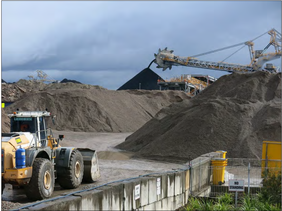
Plate 1 – General view of site in foreground. NCIG coal stacker reclaimer in background.
