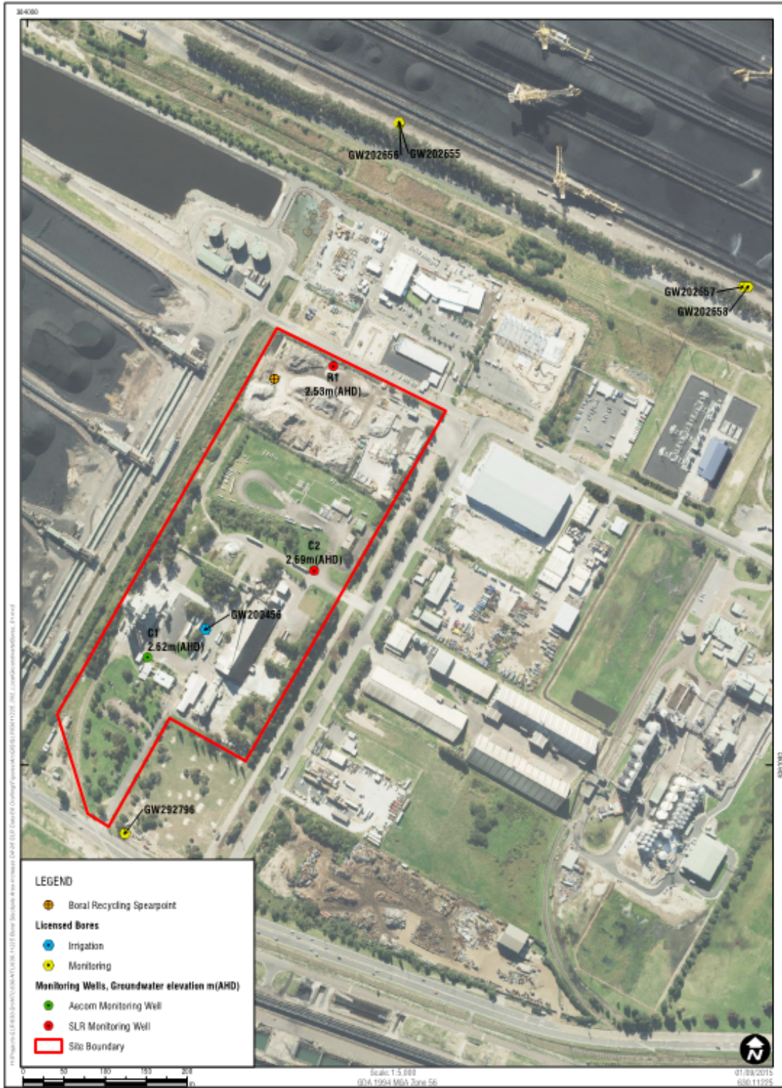
Figure 2 Groundwater monitoring well and local bore locations
