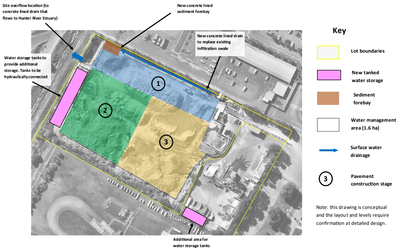
Figure 4.3 New pavement construction stages
