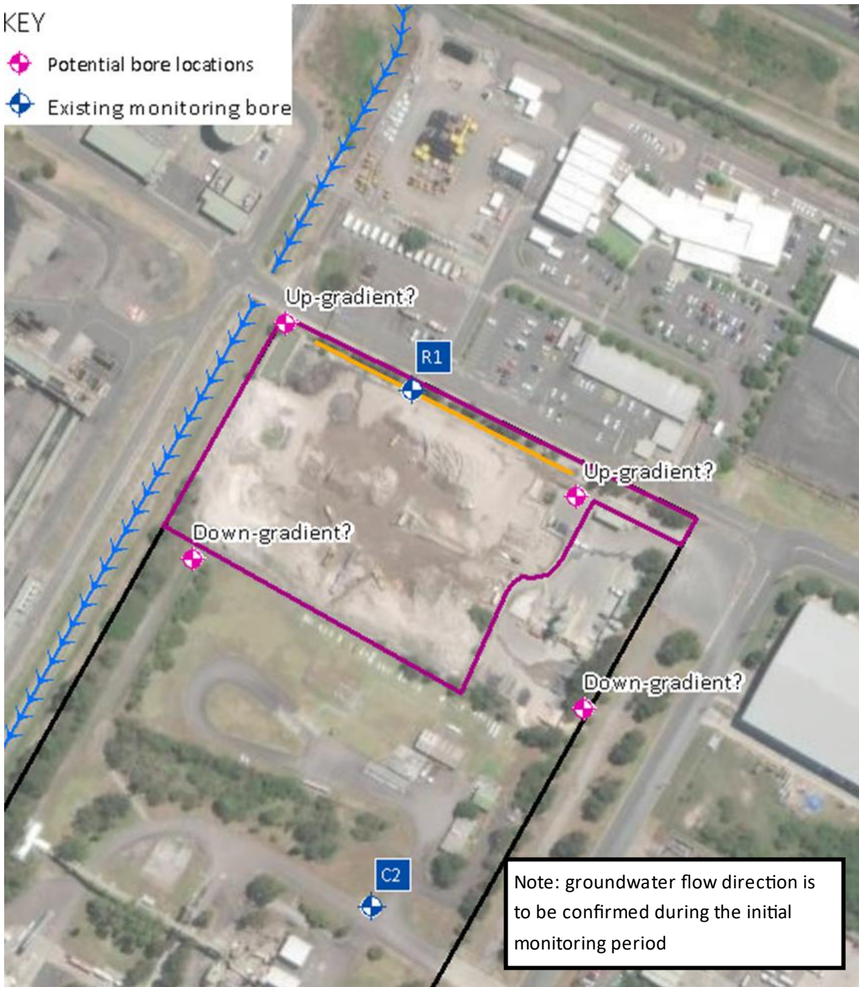
Figure 6.1 Indicative monitoring bore locations
