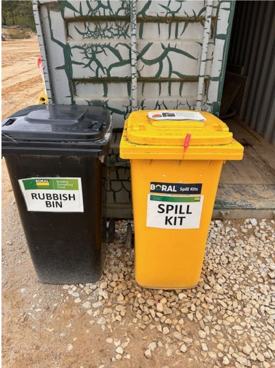
Site spill kit example with one point lesson attached to top of container
