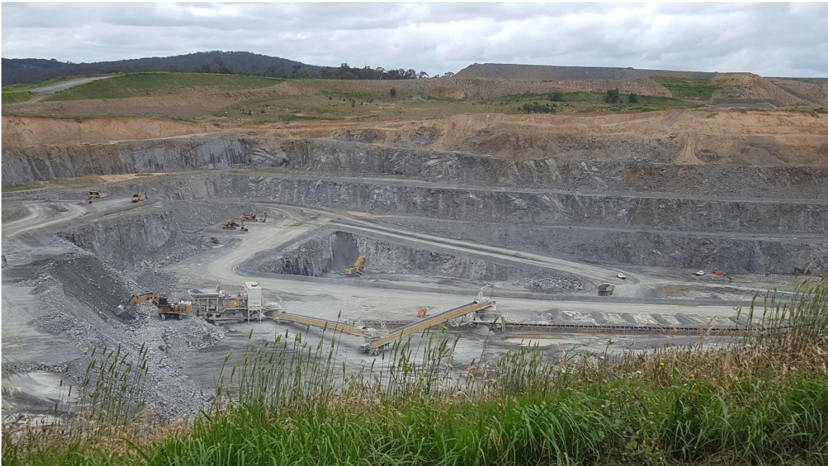
Plate 1 – Quarry Extraction Area with shaped and unshaped overburden in background
