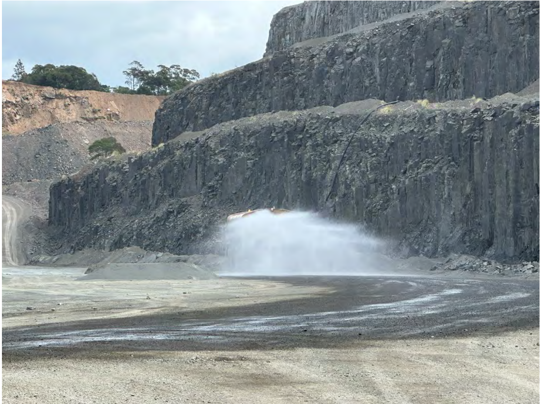
Water truck in operation on haul road.
