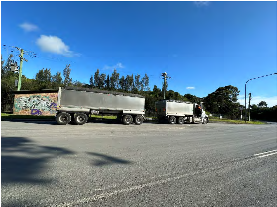
Example of covered loads when exiting the site.
