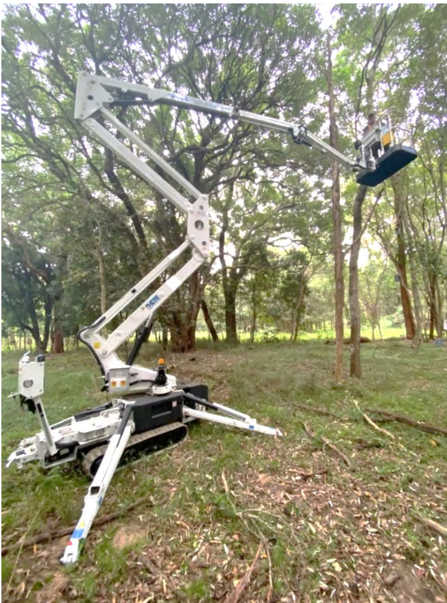
Photograph 2.1 Narrow spider lift used to install nest boxes.
