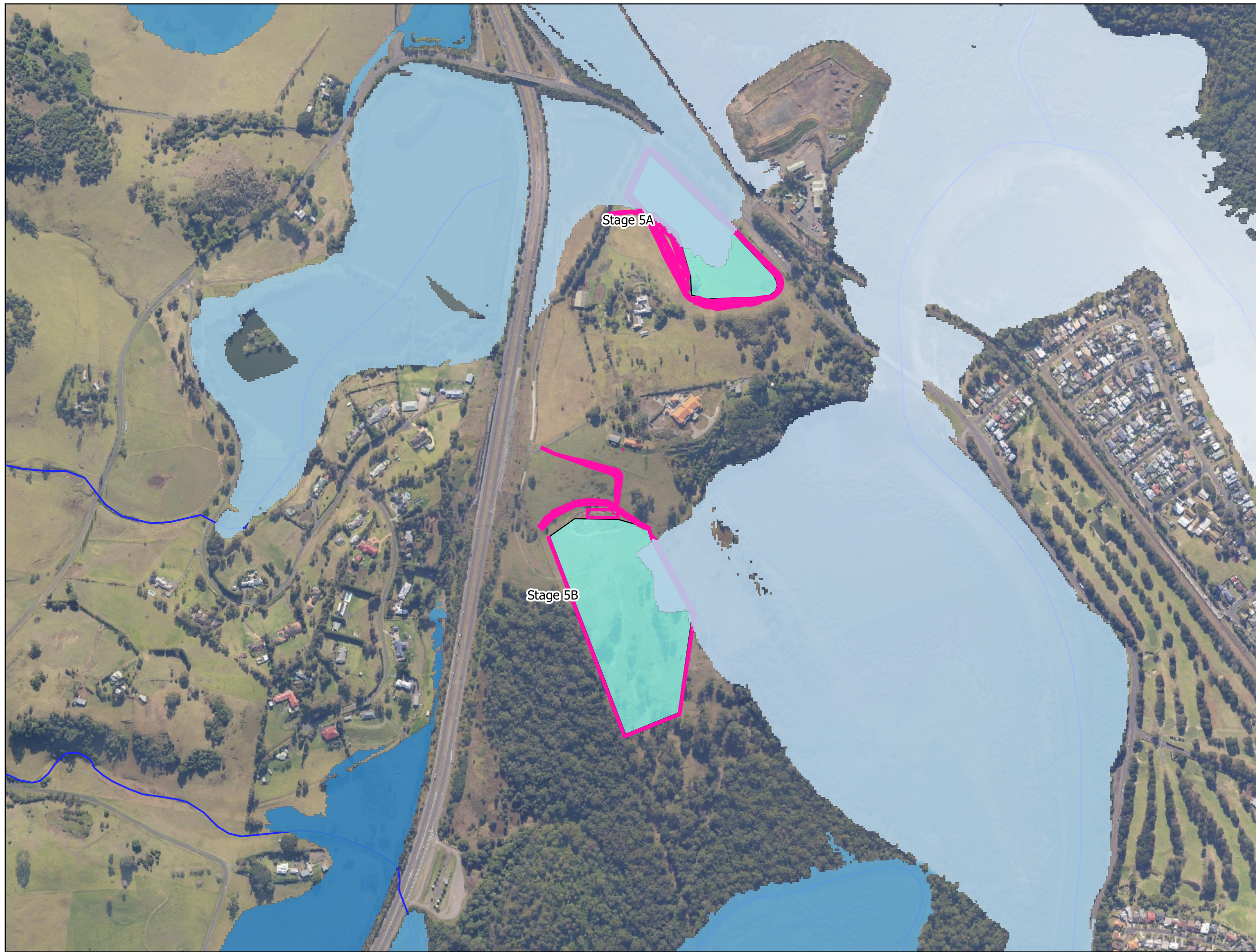
FIG 10. 20y ARI Flood height, existing conditions. 18/07/2019
