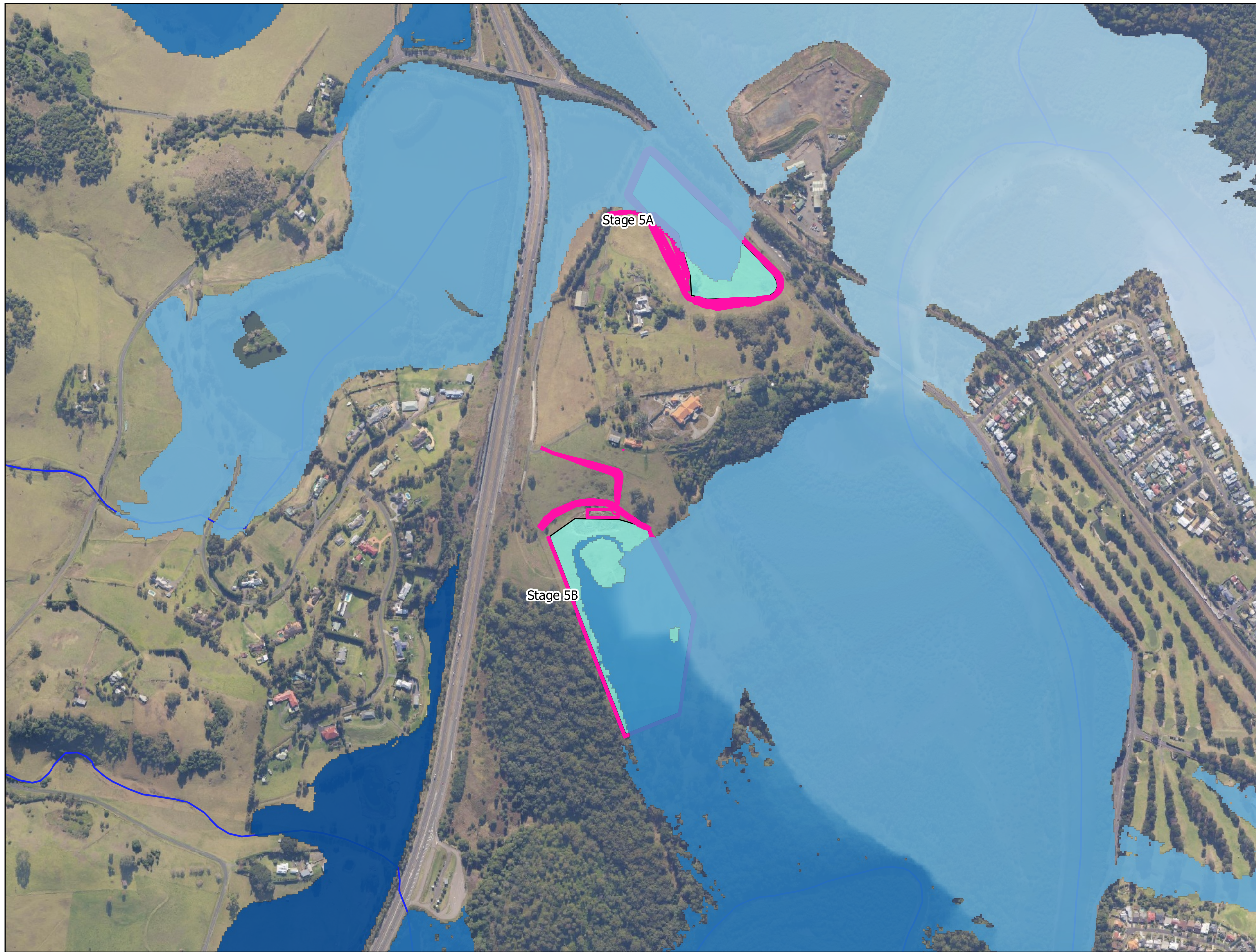
FIG 11. 100y ARI Flood height, existing conditions.
