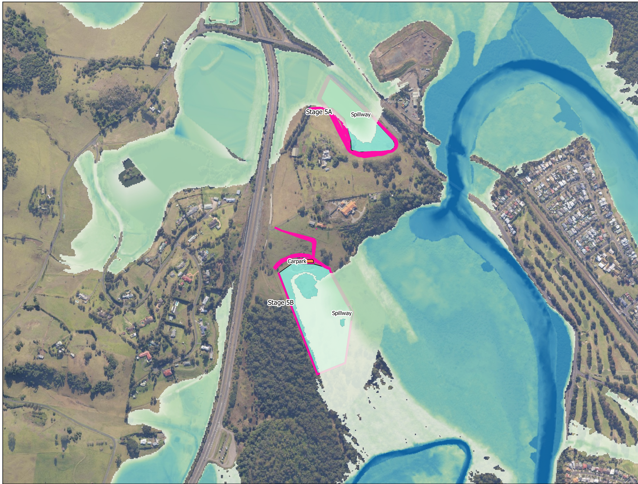
FIG 7. 100y ARI Flood depth, existing conditions.
