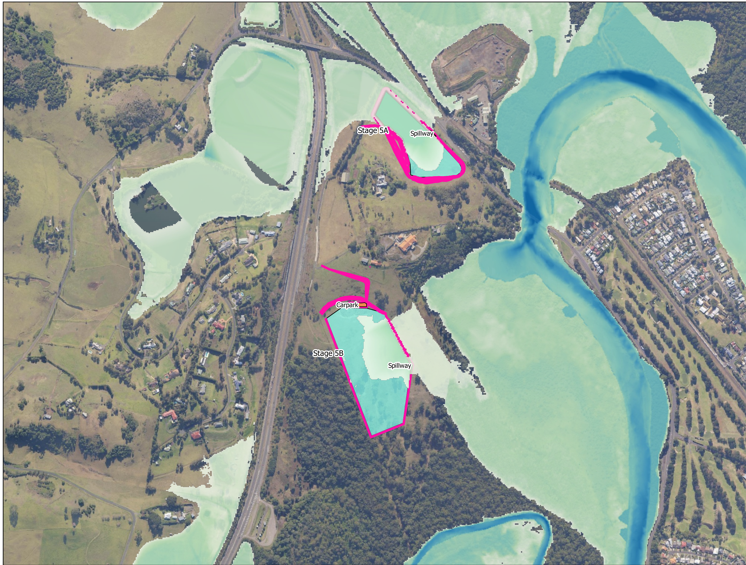
FIG 21. 5y ARI Flood depth, proposed conditions.
