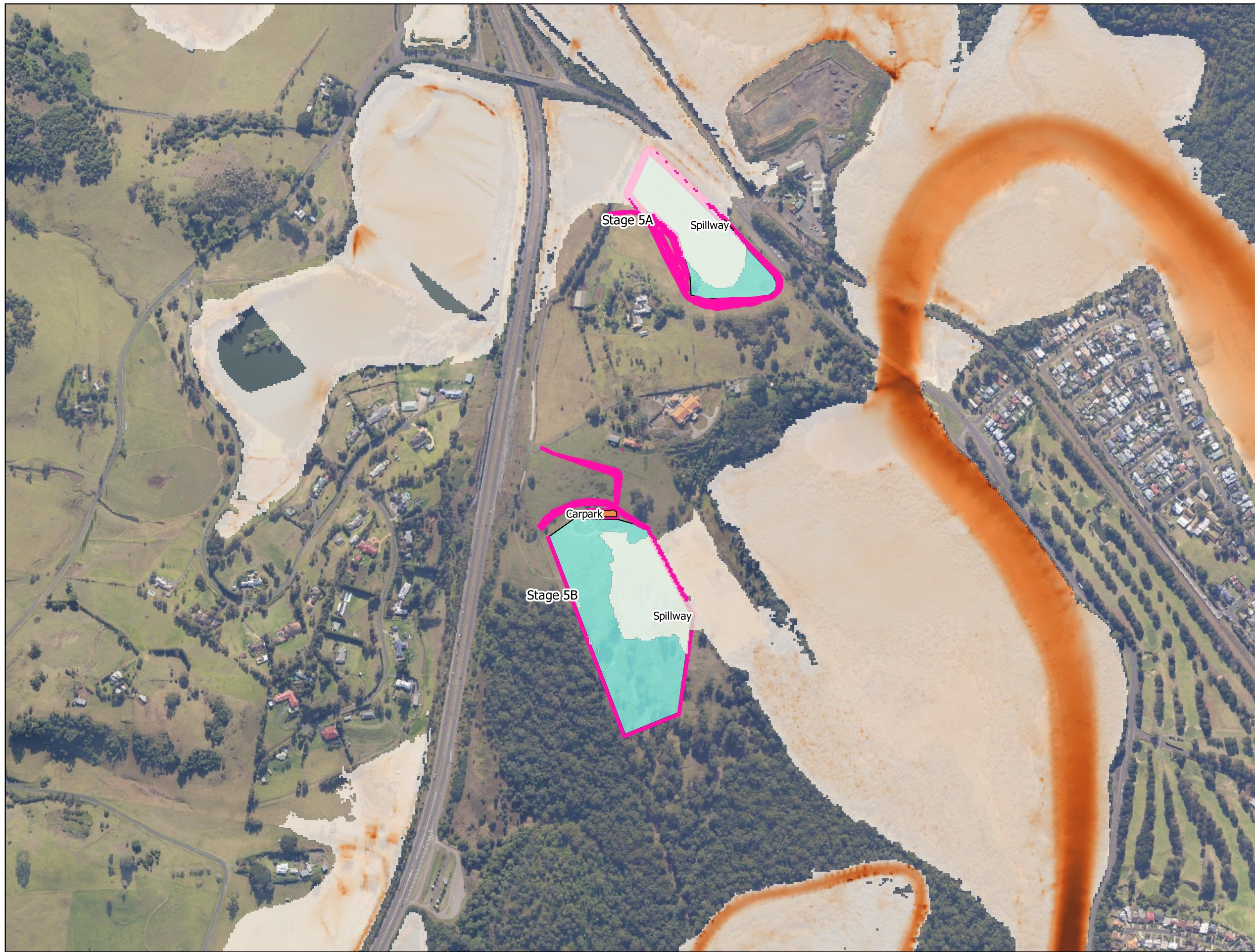
FIG 17. 5y ARI Max velocity, proposed conditions.
