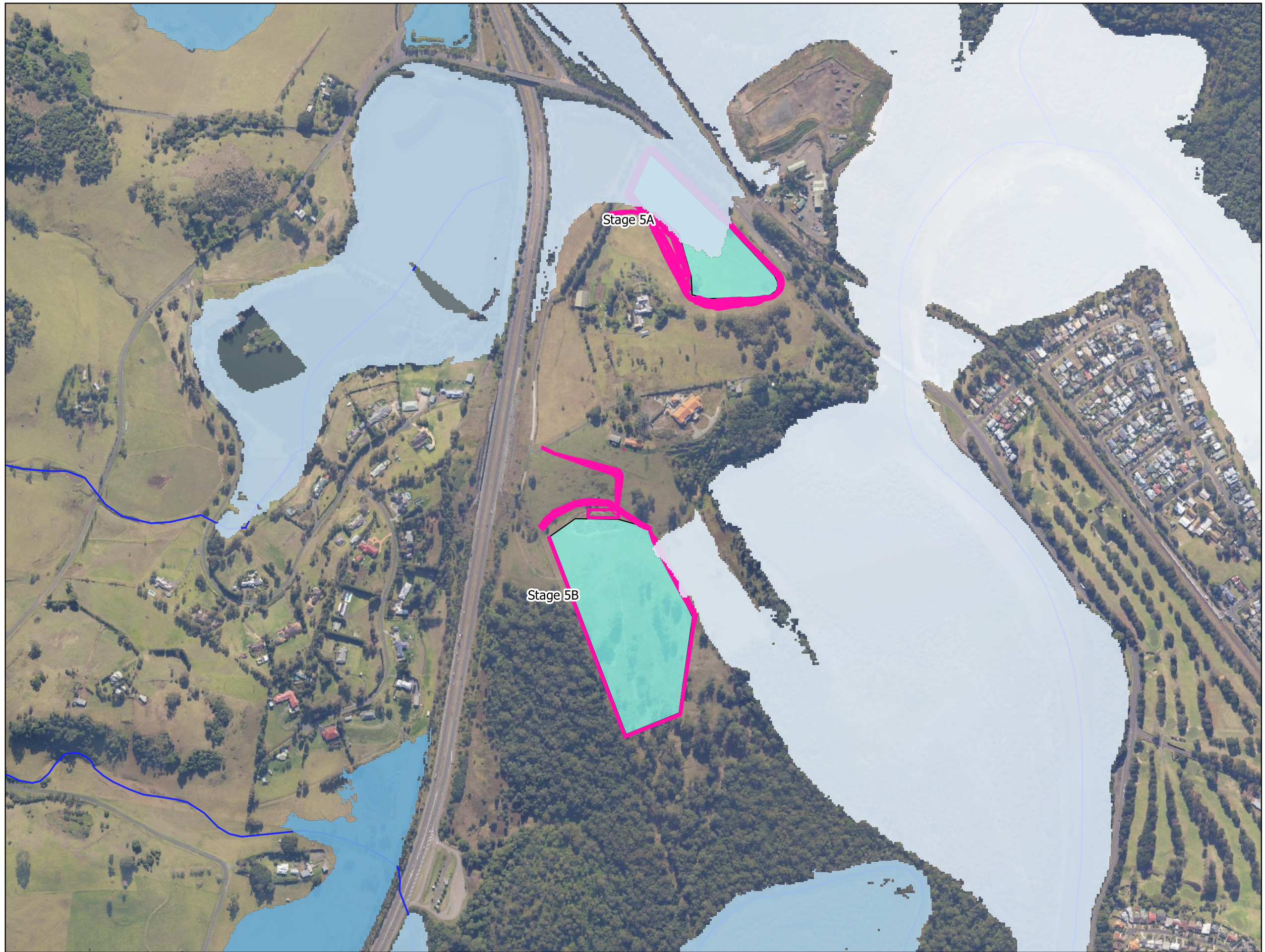
FIG 9. 5y ARI Flood height, existing conditions.
