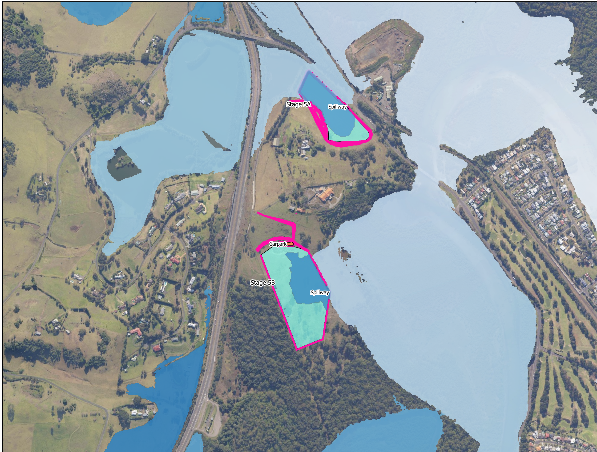
FIG 26. 20y ARI Flood height, proposed conditions.
