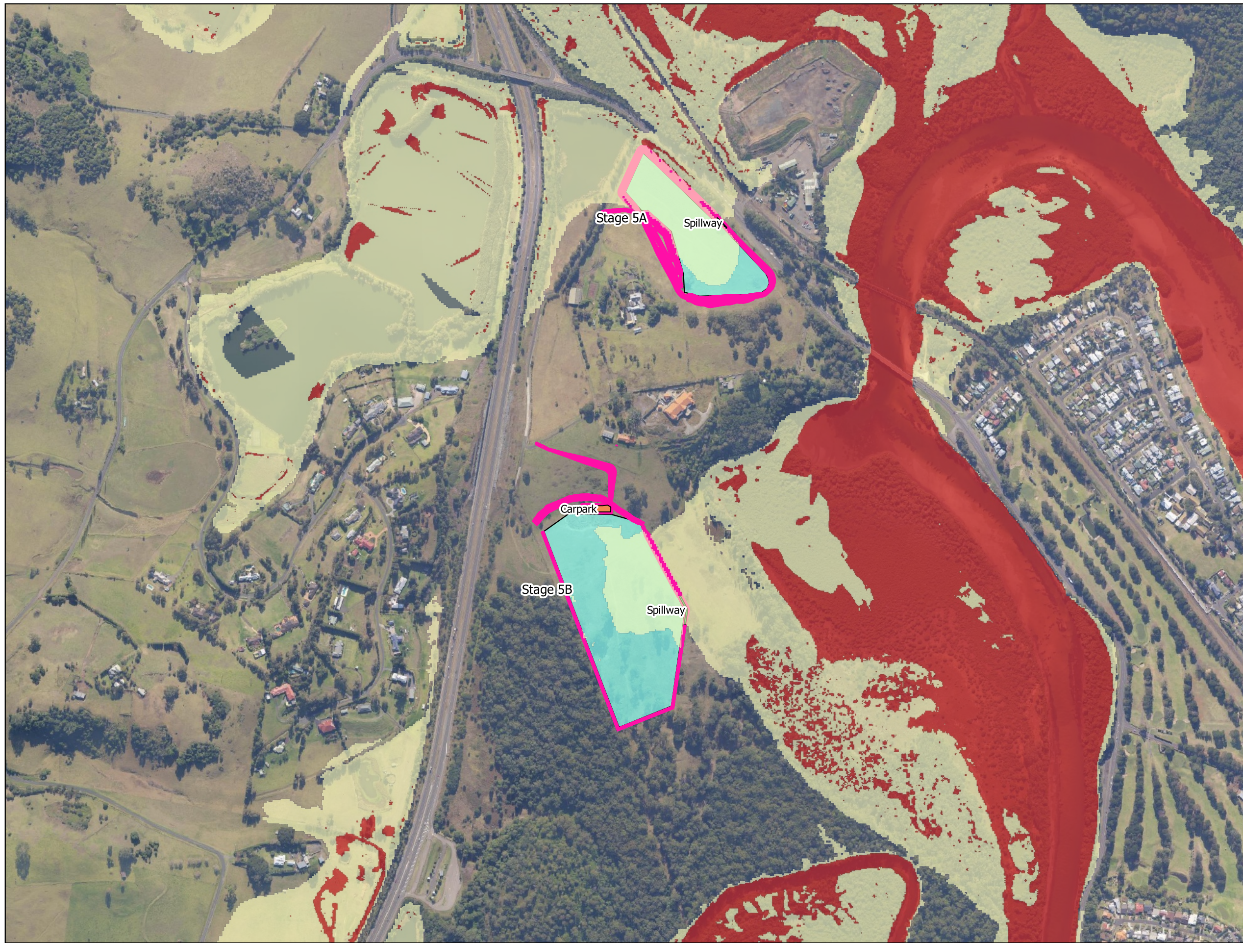
FIG 31. 20y ARI flood hazard, proposed conditions.
