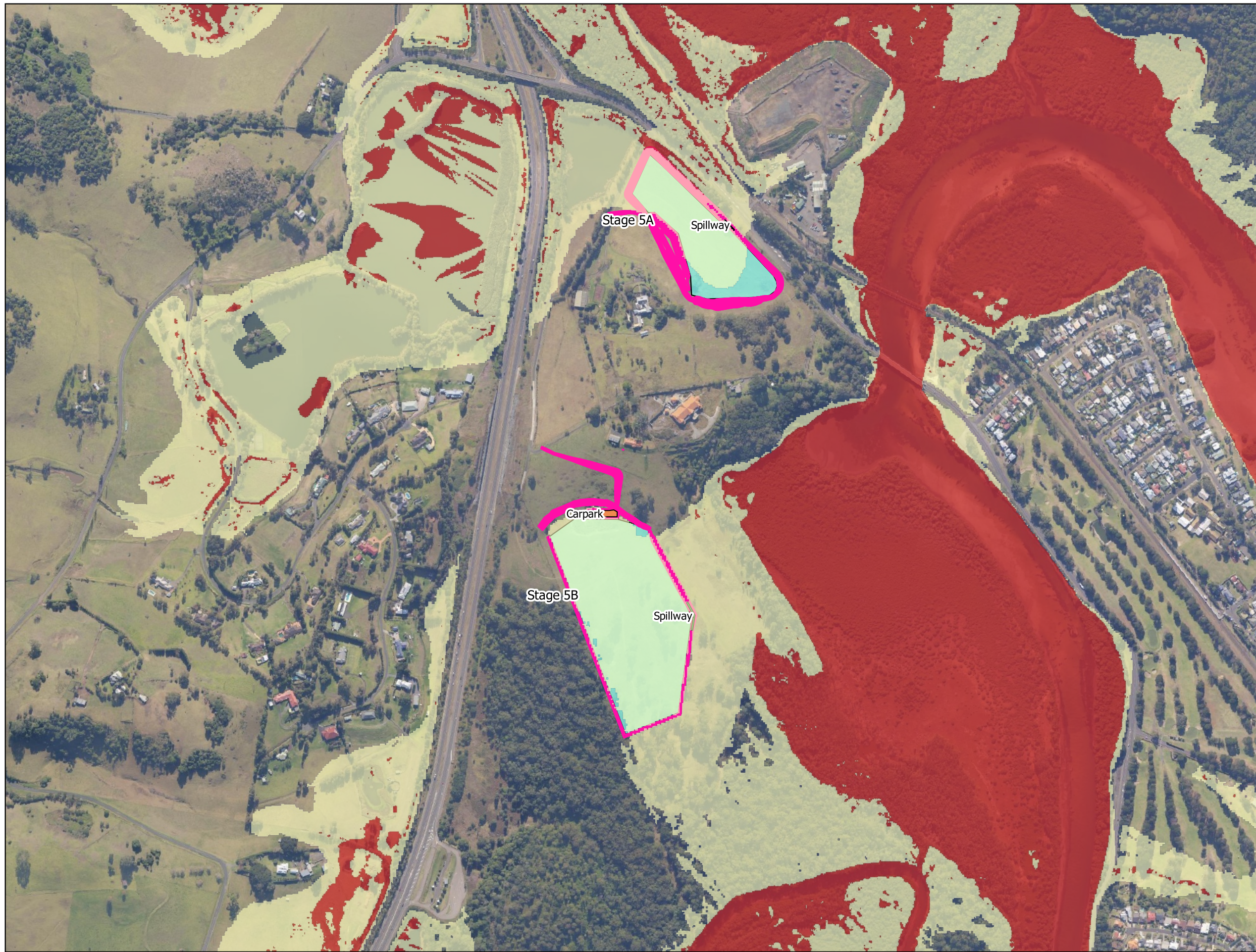
FIG 32. 100y ARI flood hazard, proposed conditions.
