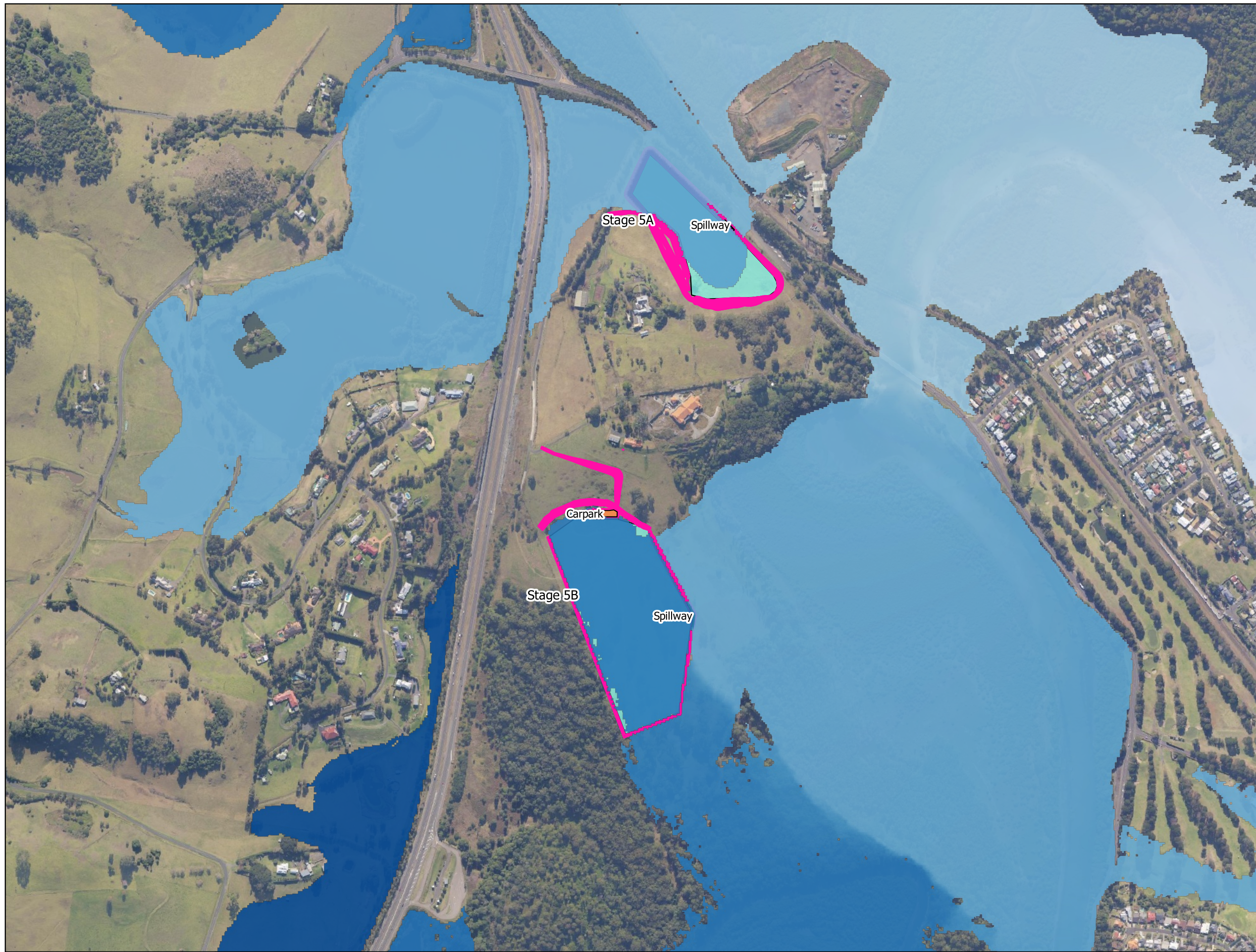
FIG 27. 100y ARI Flood height, proposed conditions.
