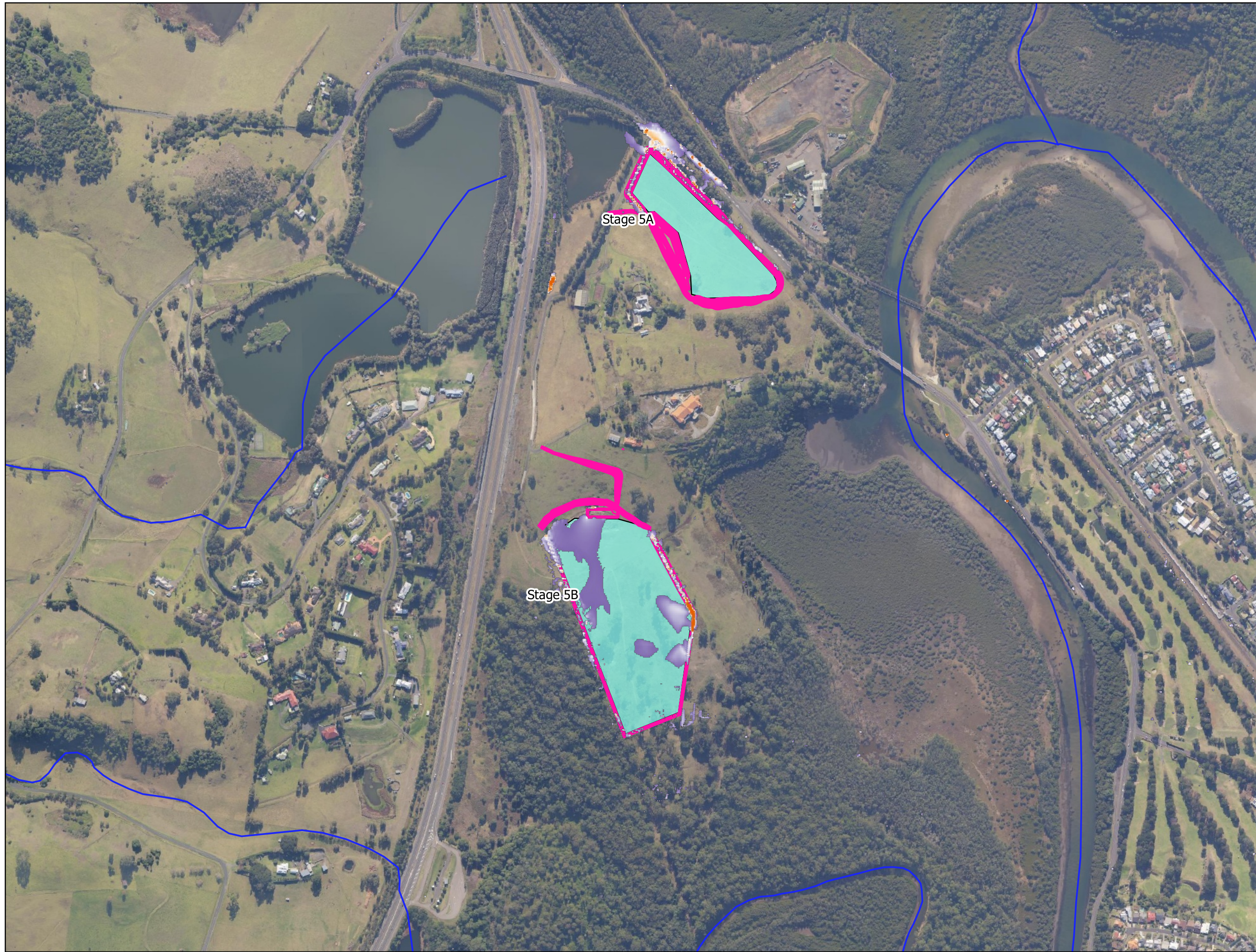
FIG 36. PMF Max velocity difference 18/07/2019
