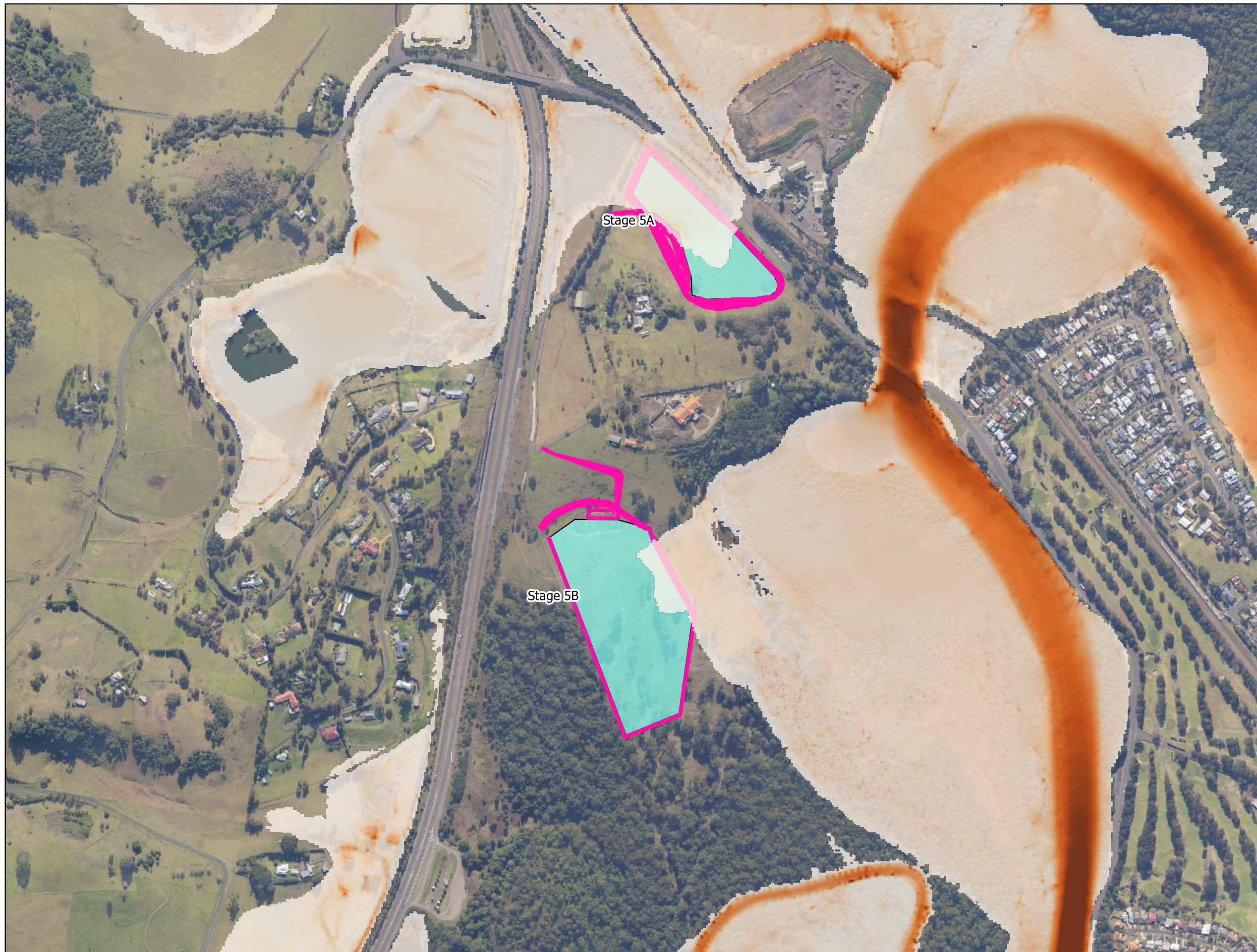
FIG 2. 20y ARI Max velocity, existing conditions.
