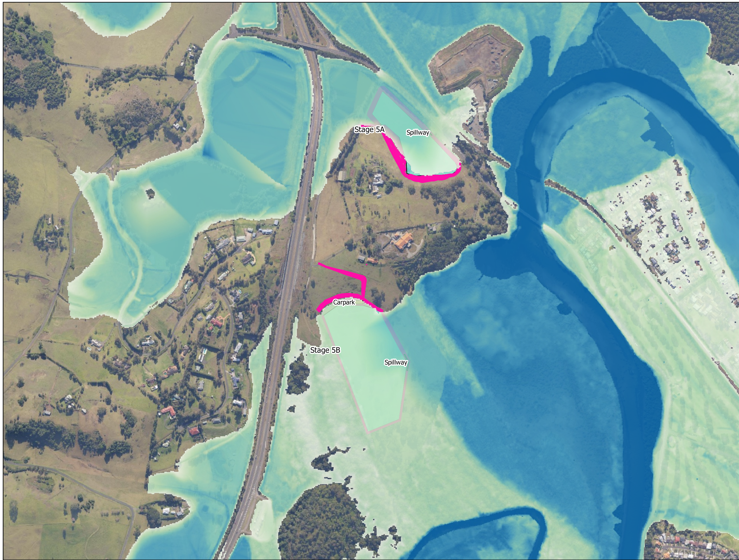
FIG 8. PMF Flood depth, existing conditions.
