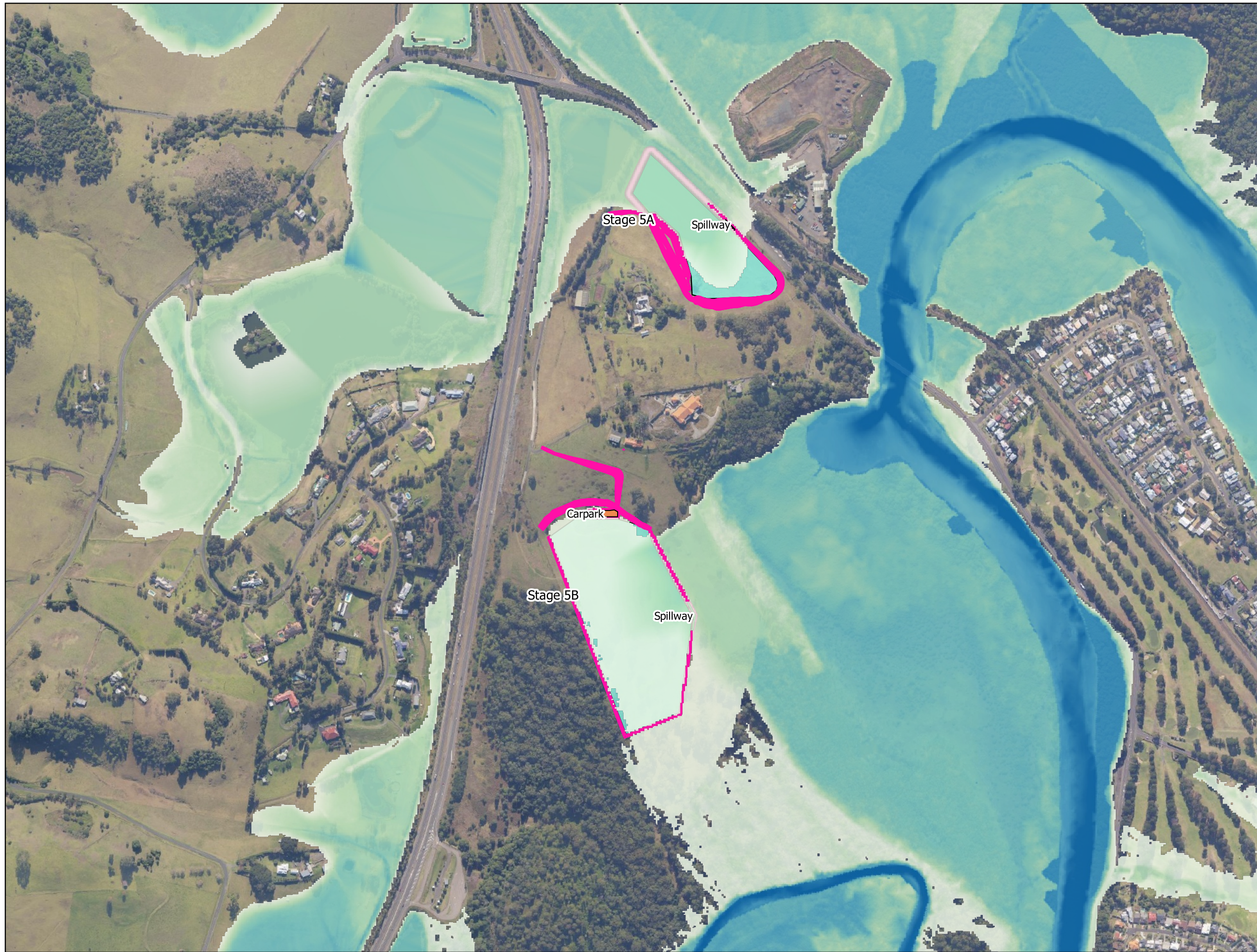
FIG 23. 100y ARI Flood depth, proposed conditions.
