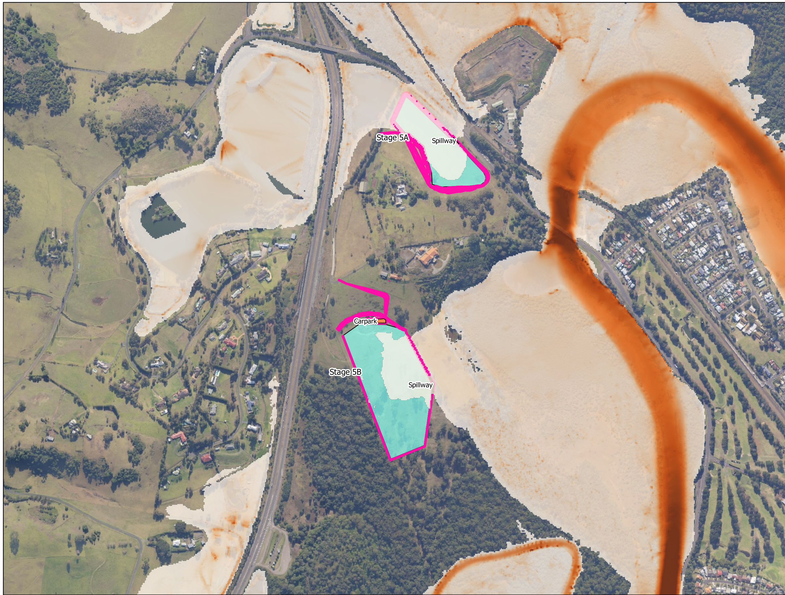
FIG 18. 20y ARI Max velocity, proposed conditions.
