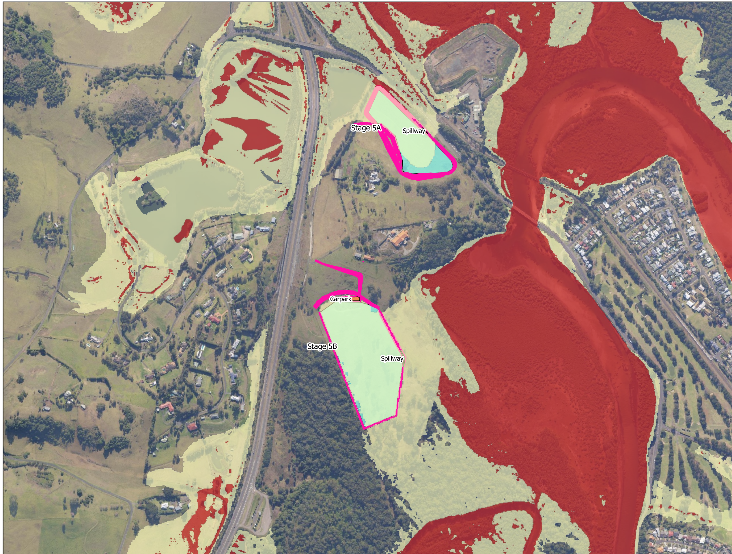
FIG 24. PMF Flood depth, proposed conditions.
