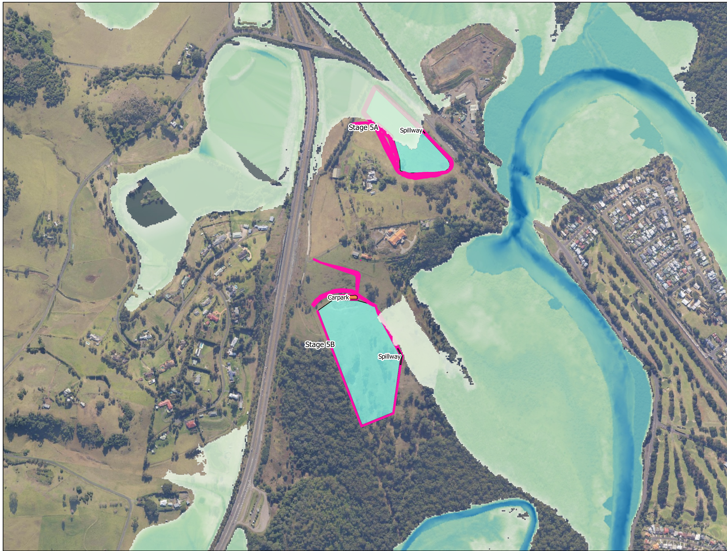
FIG 5. 5y ARI Flood depth, existing conditions. 18/07/2019
