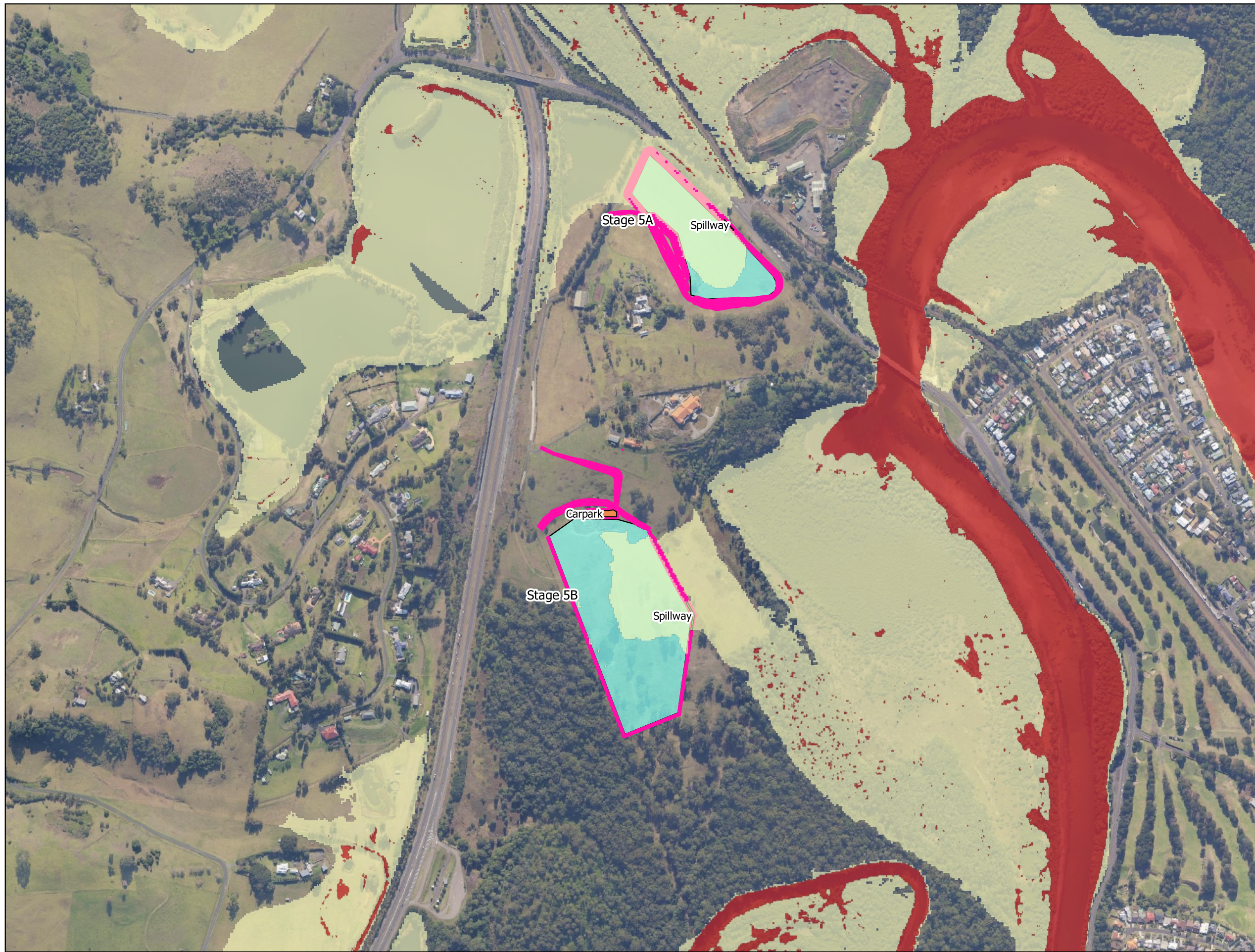
FIG 30. 5y ARI flood hazard, proposed conditions.
