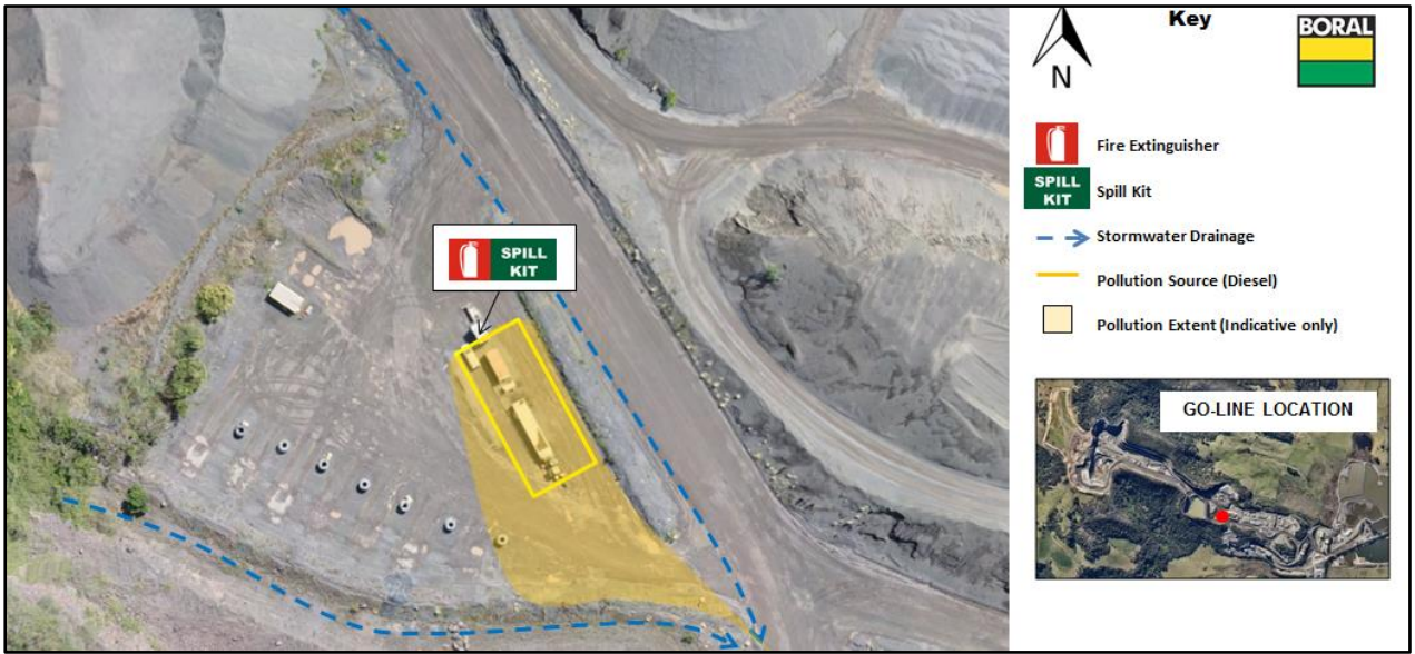
Figure 3: Go-line Above Ground Diesel Storage Area
