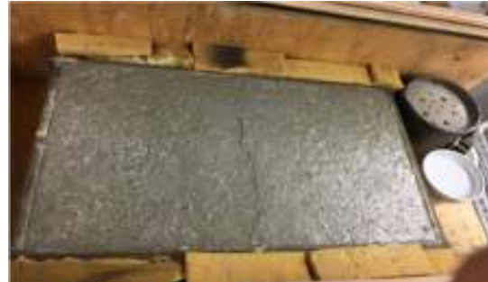
Figure 2 (b) – ASTM environmental chamber including set time sample and evaporation dish
